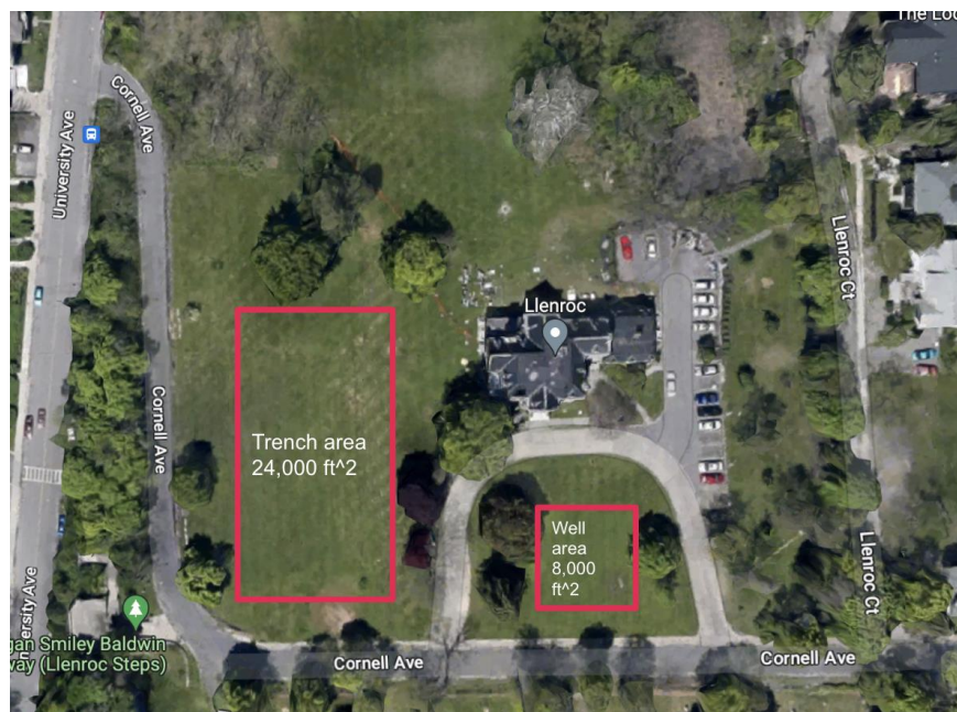
Figure 14: Areas of trenches and wells for heat pump in Llenroc's yard
