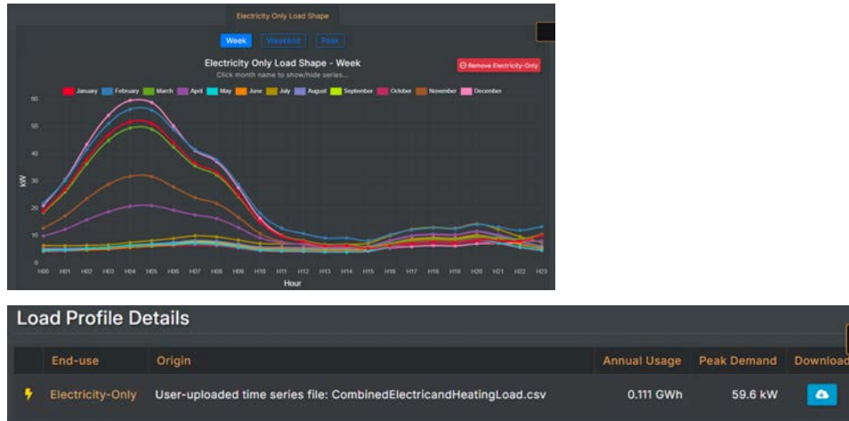
Figure 9. Combined heat and electric load profile
