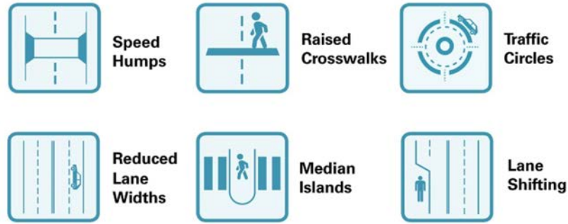
Figure 2: Typical Traffic Calming Devices
