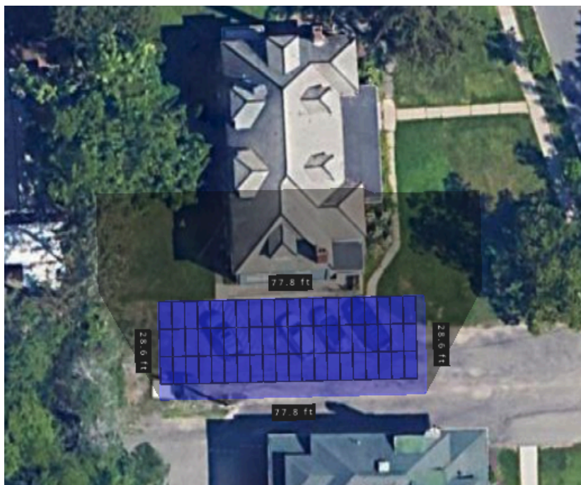
Figure 5: Helioscope Design of Solar Parking Canopy
